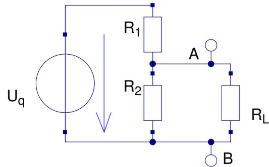
$$U_q = 5V, R_1 = 1k\Omega, R_2 = 5k\Omega$$
