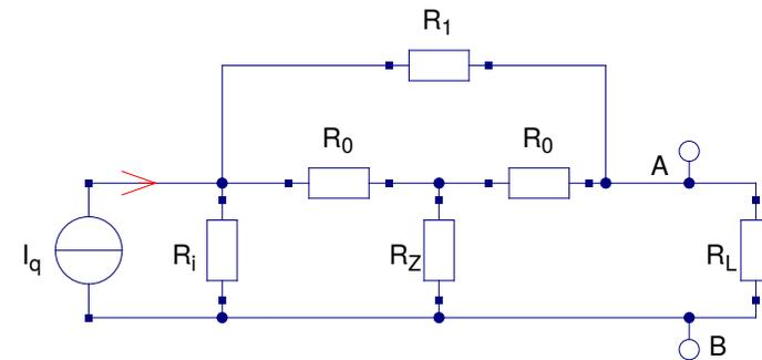
$$I_q = 10mA, R_i = 50k\Omega, R_0 = 5\Omega, R_1 = 10\Omega, R_Z = \frac{R_1^2}{R_0}$$
